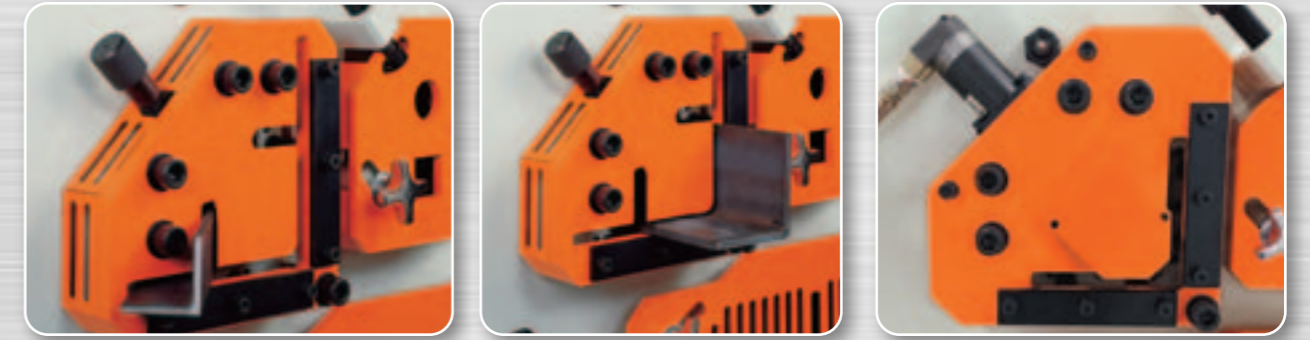
*Optional hydraulic hold-down for angle shear.
